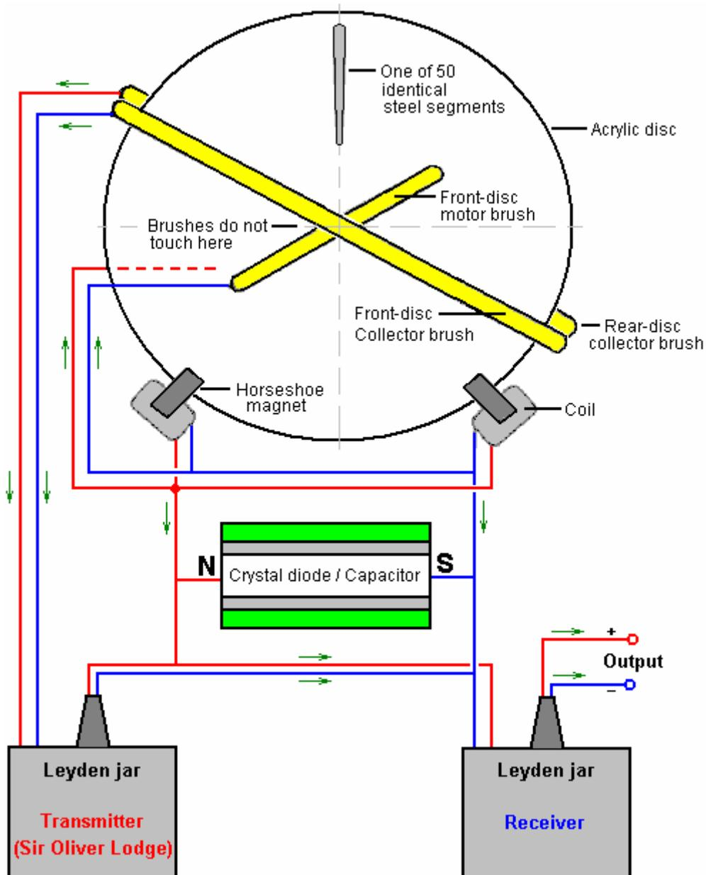
The collector brushes on the front and rear faces of the spinning disc collect charge and although the design has never been disclosed, it has a constant power output: of 300 volts at 10 amps which is 3 kilowatts. So much for electrostatic electricity being only trivial !!
