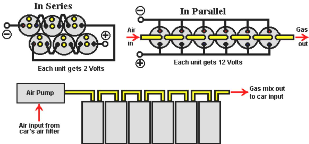
The air connection is the same for either method of wiring the cells. If wired in series, the voltage drop across each cell may not be the same although they were constructed in an identical fashion.
