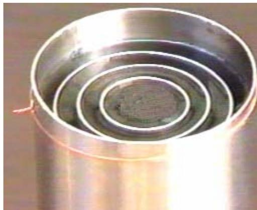
The picture above shows the general construction of a cell of this type although, unlike the description below, this one does not have the lip which is used for attaching the lid. It is included here just as a general illustration of how the cylinders are positioned relative to each other.
