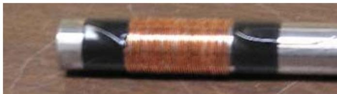
The wire for the second layer is cut to a length of 396 centimetres. This second coil layer will be longer than the first layer, so before winding it, it's necessary to build up the area at both ends of the first layer with tape:
