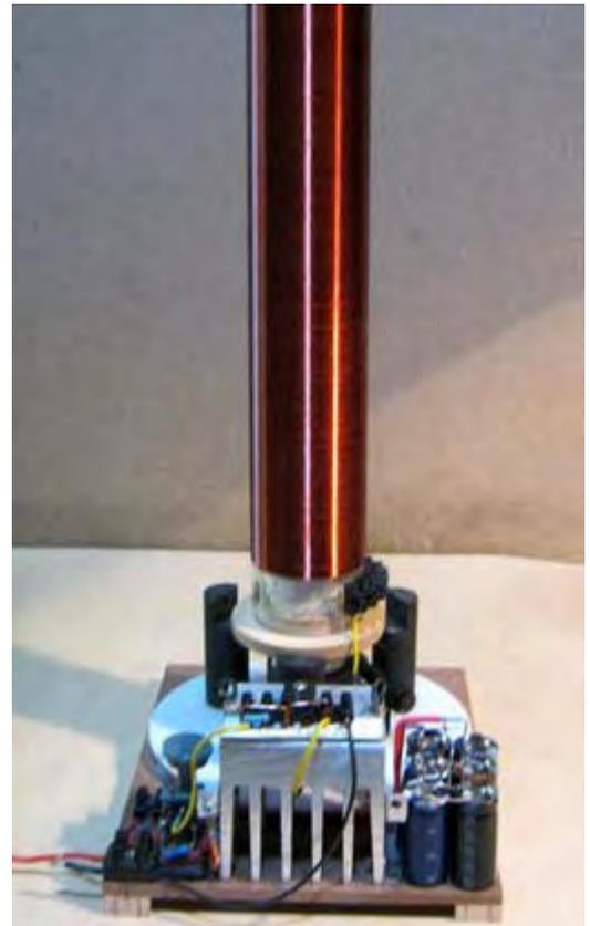
I am using a TIP3055 transistor. I have tried a range of transistors, MJE13009, TIP132 and all sorts of others, and the only one's which work at all are the 2SC3552 (1000V) and the TIP3055, which is the best by far.
