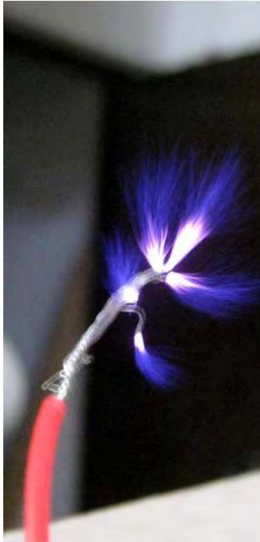
I then measured the voltage at L2 empirically, and found it able to charge a 1 microfarad capacitor rapidly to 2,000V. I presume the rectified AC voltage to be far higher, at least in the multi-kilovolt range. I feel that the formula mentioned by Solovey,  $U_2 = U_m / N_1.N_2$ , does not necessarily apply to this type of Tesla configuration, so I question his calculation of 700-800V.
