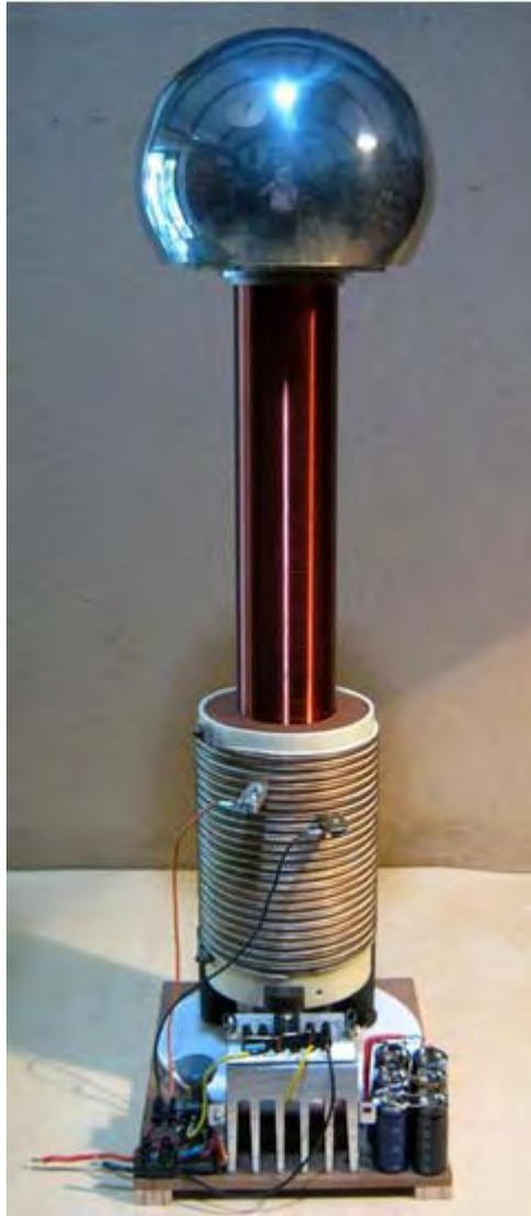
I was also able to dispense with the 100 ohm resistor, as the current draw from the 12V supply battery was now down to 2 amps, which is much more reasonable, but still more than Solovey's 0.3 amps.
