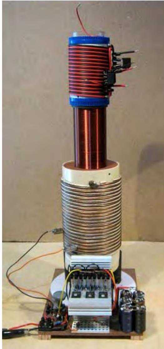
I have vertically flipped coil L1 so that the 3 active windings are now at the bottom, and moved the pickup L3 right to the top of L2. I also noticed that the output in this configuration increased substantially when I removed the aluminium globe and just left the open end of the Perspex tube at the top of L2. This is good news as these metal spheres are not easy to find.
