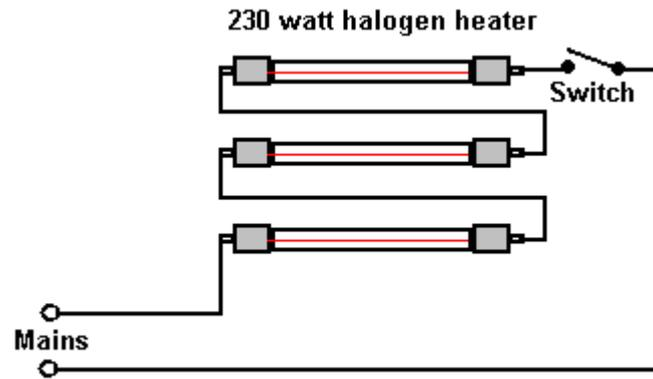
If the halogen heater is now connected across 700 volts, the result is that if the halogen bulbs are similar to each other, then about one third of the 700 volts will be across each bulb. This is only an untested suggestion although a heater of this type works well at low power on 220 volts, but it gives a high voltage resistive load as a starting point for experimenting.
