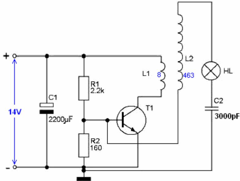
**Fig. 6.** Schematic: inserting an incandescent lamp in series through L2 and C2.
