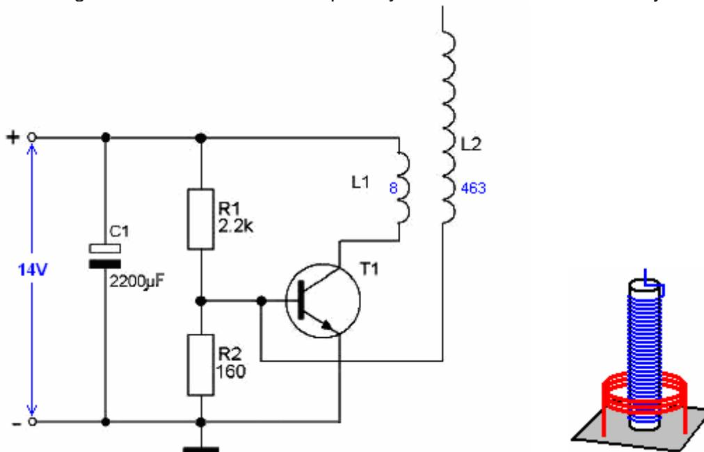
**Fig. 2.** Schematic of windings L1 and L2
