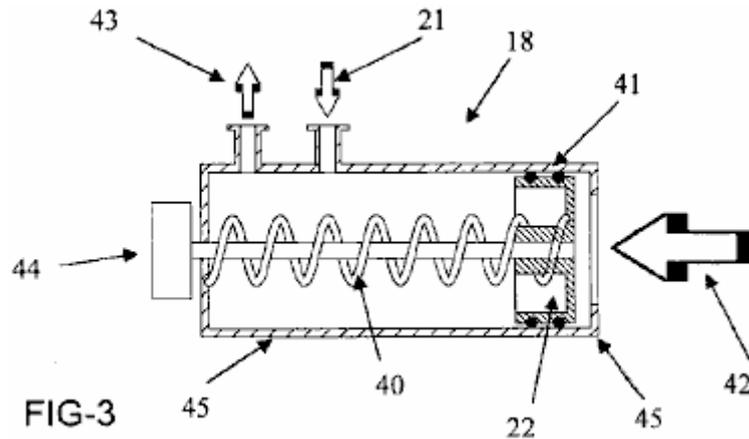
**Fig.3** shows one version of the first air reservoir **18**. Air is drawn into reservoir **18** through air intake **21**. The reservoir includes a piston **22** associated with a spring **40**, the piston **22** being provided with seals **41** to prevent leakage of air.
