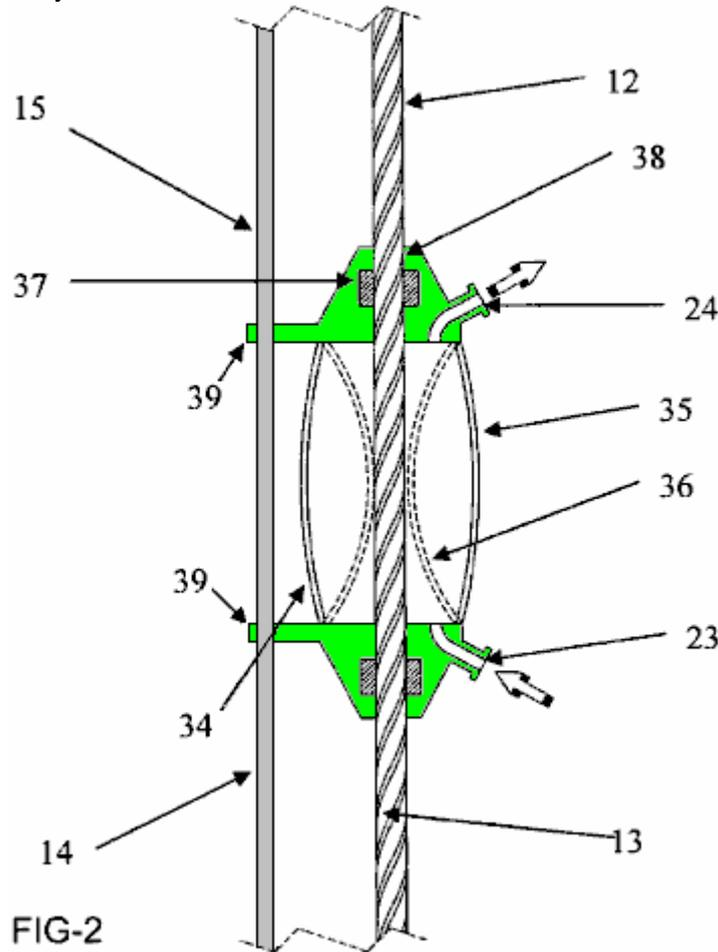
**Fig.2** shows one arrangement for buoy 14 comprising an inflatable capsule 34. This figure illustrates the shape of the walls of the inflatable capsule 34 when inflated 35 and when deflated 36. Air passes into capsule 34 through hose 23 and exits from the capsule through hose 24.
