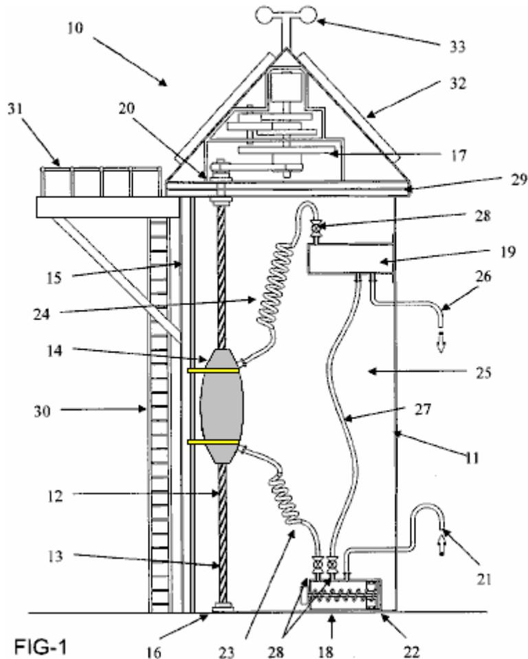
**Fig.1** is a cross-sectional view of an embodiment of the energy generation system of the present invention. Here, the energy generation system **10** comprises a vessel **11** in the form of a water tank and a shaft **12** which can rotate about its longitudinal axis. The shaft **12** is provided with a helical screw groove **13** and is connected at its lower end to a bearing **16** which allows it to rotate freely about its longitudinal axis.
