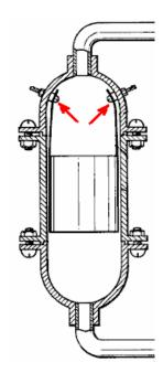
Next, two powerful permanent magnets are mounted in the container, one above the electrodes and one below them:
