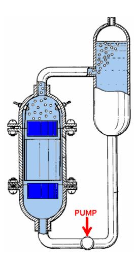
The output pipe of the electrolyser is connected to the side of the electrolyte reservoir and there, the bubbles float upwards and exit through a bubbler while the remaining electrolyte gets circulated again by the pump.
