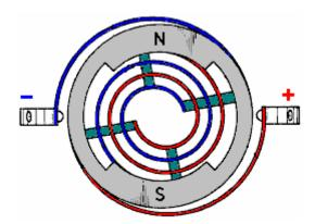
The magnets are arranged to produce a magnetic field which runs across the axis of the electrolyser. The spacers (shown in green) are not continuous but are quite separate, and they are there to cause turbulence as well as to force the desired electrode spacing:
