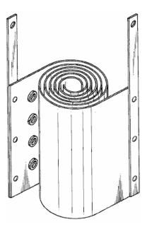
These electrodes are surprisingly difficult to make by hand but they should be very simple to construct using a 3D printer. These electrodes are then bolted to a non-conducting enclosure:
