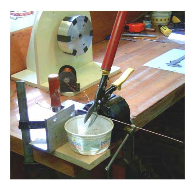
THE DISTANCE BETWEEN THE SHEARS AND THE METAL CLAMPED TO THE WORKBENCH MAKES EACH CUT LENGTH OF WIRE EXACTLY THE SIZE REQUIRED, WHILE THE PLASTIC CONTAINER COLLECTS THE CUT PIECES READY FOR COATING WITH CLEAR SHELLAC OR WITH CLEAR POLYURETHANE BEFORE USE IN THE COIL CORES.
