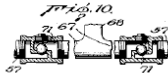
Fig.9 and Fig.10 are detail sectional views showing the inlet and outlet to the cylinders of the atomising pump.
