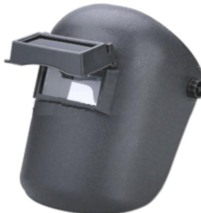
This type has a clear glass screen and a hinged safety filter to allow safe welding. Professionals adjust the hinge tension so that the filter can only just stay in its raised position. The welder then positions the joint pieces in their exactly correct position while looking through the plain glass, and when ready to start the weld he just nods his head which makes the filter drop into place and the weld is started. Never, ever, try welding without proper eye protection
