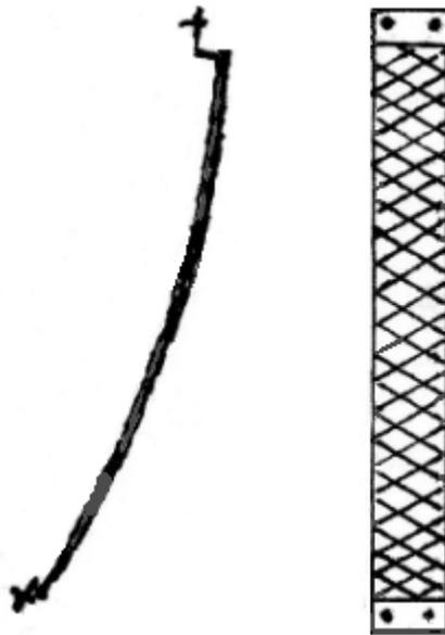
This strip is bolted or welded to just one point on the rim of the main flywheel like this:
