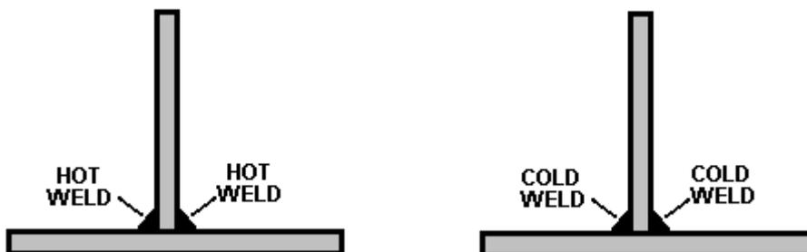
Then, as the welds cool down, they pull in opposing directions and while it produces stresses in the metal, the vertical piece stays vertical. Let the welds cool down in their own good time, taking perhaps ten minutes to cool properly. Do **not** apply water to the welds to speed up the cooling as that actually alters the structure of the steel and you really don't want to do that.
