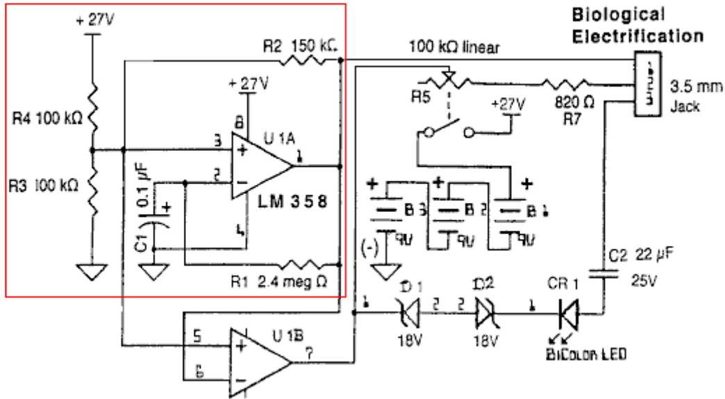
Bob states that the first section acts as a 4Hz square-wave signal generator, the frequency being controlled by the 2.4M resistor "R1" and the 100nF capacitor "C1". The data sheet for the LM358 states that the output voltage swing is between zero volts and 1.5V less than the supply voltage "Vcc" (which is +27V in this case). That implies that, as would be expected, the pin 1 output voltage from the first stage will switch sharply from 0V to +25.5V and sharply back again, four times per second.
