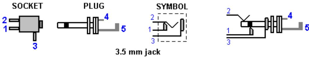
When the plug is not inserted into the socket, pin 1 connects to pin 2 and pin 3 is not connected to anything. When the plug is inserted, then pin 1 is isolated, pin 2 is connected to plug pin 4 and pin 3 is connected to plug pin 5.
