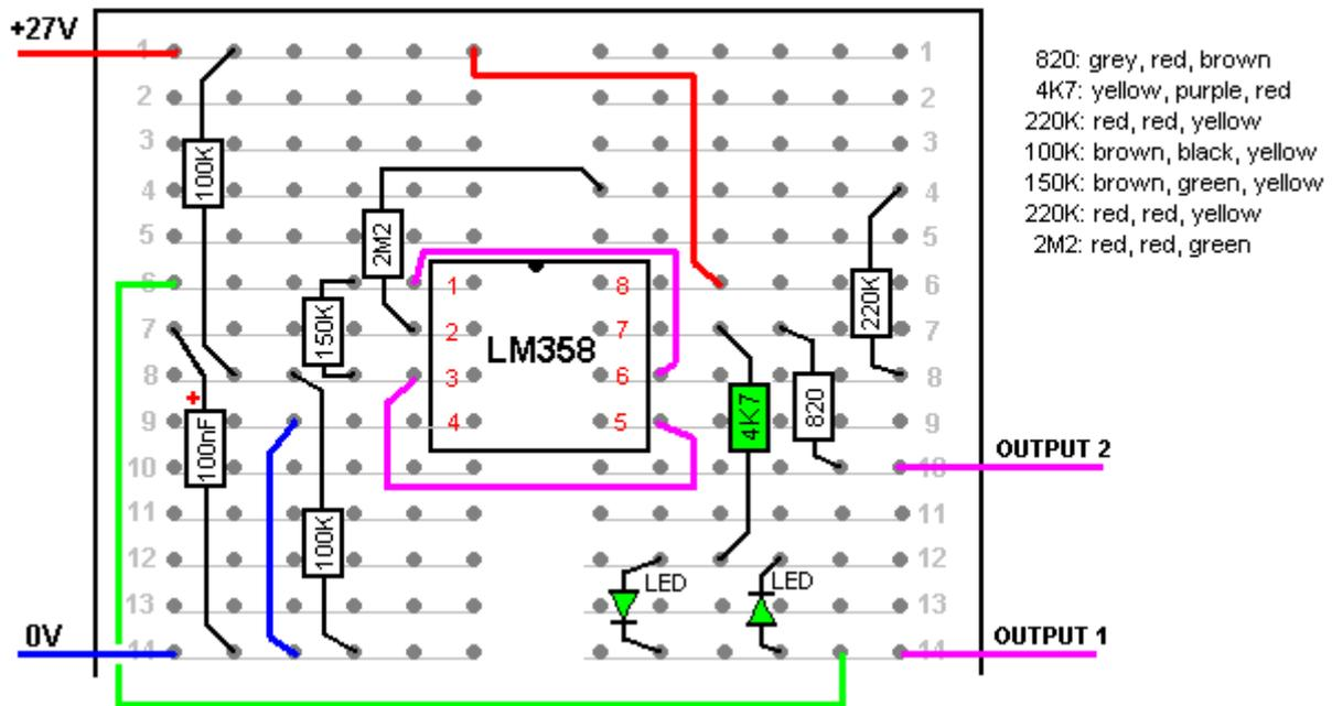
The 4.7K resistor and LEDs are only on the board for testing purposes and when the circuit is built in permanent form, then the LED chain connects to pin 1 of the jack socket so that the LEDs are disconnected during the two hours of daily treatment recommended when using the device.
