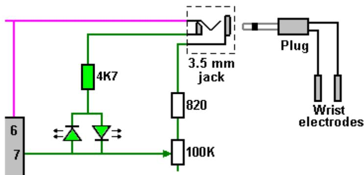
With this arrangement, the two LEDs flash alternately. In any circuit, a capacitor with a higher voltage rating can always be used if the capacitance values are the same. The Beck external circuit is completed through the body of the user, so there is just one electrode connected to each side of the output jack socket.
