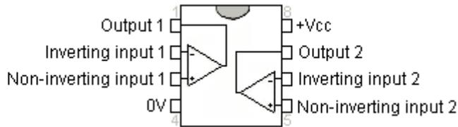
This chip draws only half of one milliamp, has two very high-gain operational amplifiers and can operate with a wide range of supply voltages. It is also inexpensive.
